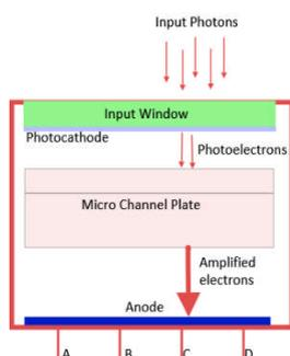
*Diagram 1. Structure of IPD Detector*
