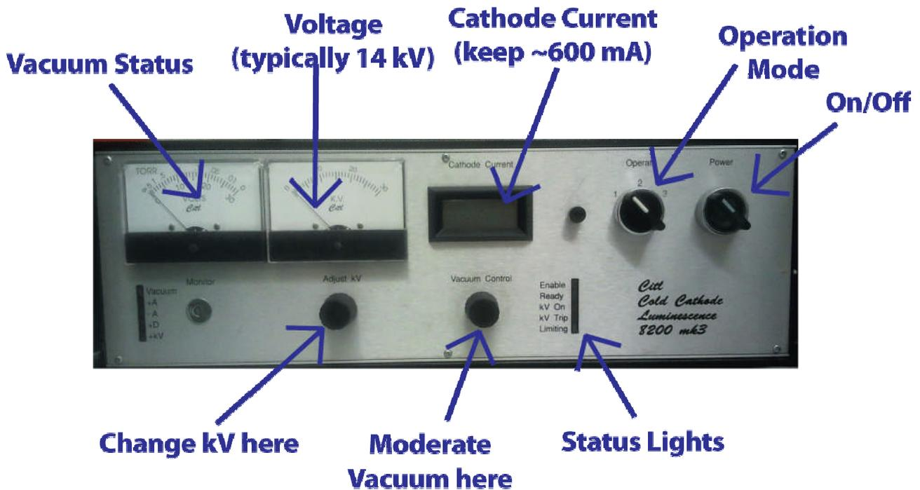
**Figure 2:** Front Panel of the Control System (Luminoscope)
